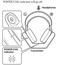
About the charging method of the system This system employs a contactless charge method that requires no terminals by the electromagnetic induction.
